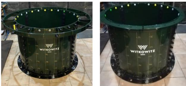
FIGURE 1 ASSEMBLED PROTOTYPE, LEFT WITH NWG AND RIGHT WITH STANDARD GIRDER L60
