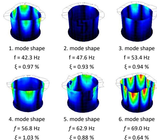
FIGURE 5 MODE SHAPES OF STORAGE TANK WALL WITH NWG
