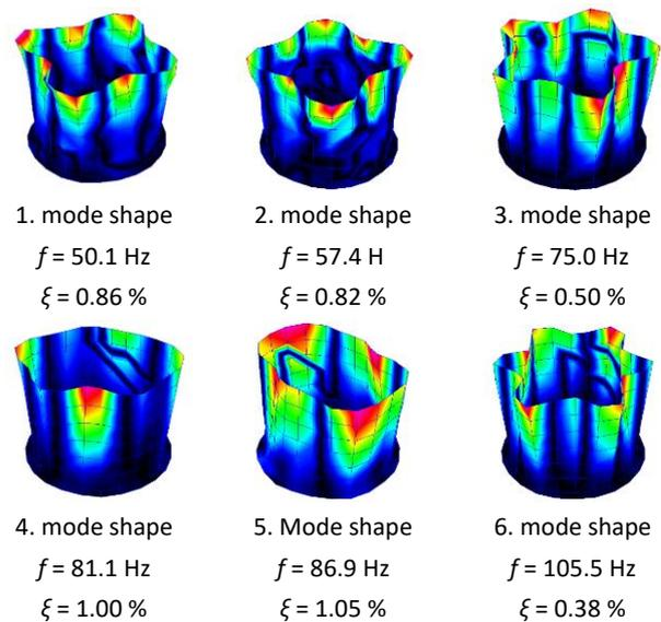
FIGURE 3 MODE SHAPES OF STORAGE TANK WALL WITHOUT GIRDER
