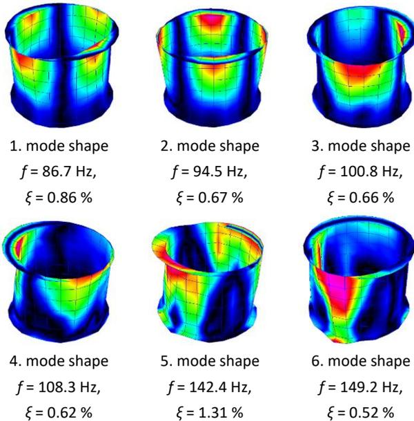
FIGURE 6 MODE SHAPES OF STORAGE TANK WALL WITH STANDARD GIRDER L60
