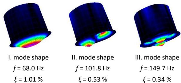
FIGURE 4 MODE SHAPES OF STORAGE TANK BOTTOM
