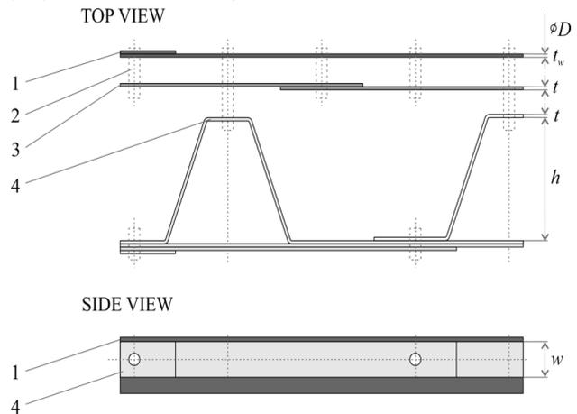
FIGURE 2 SHAPE OF SEGMENTS FORMING NWG: ITEM 1: TANK WALL, ITEM 2: BOLTED CONNECTION, ITEM 3: P-SEGMENT, ITEM 4: V-SEGMENT
