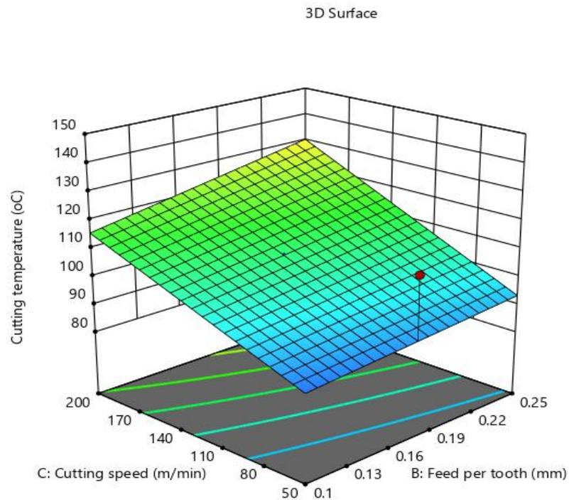
Figure 6. Effect of DOC and CS on cutting temperature.
