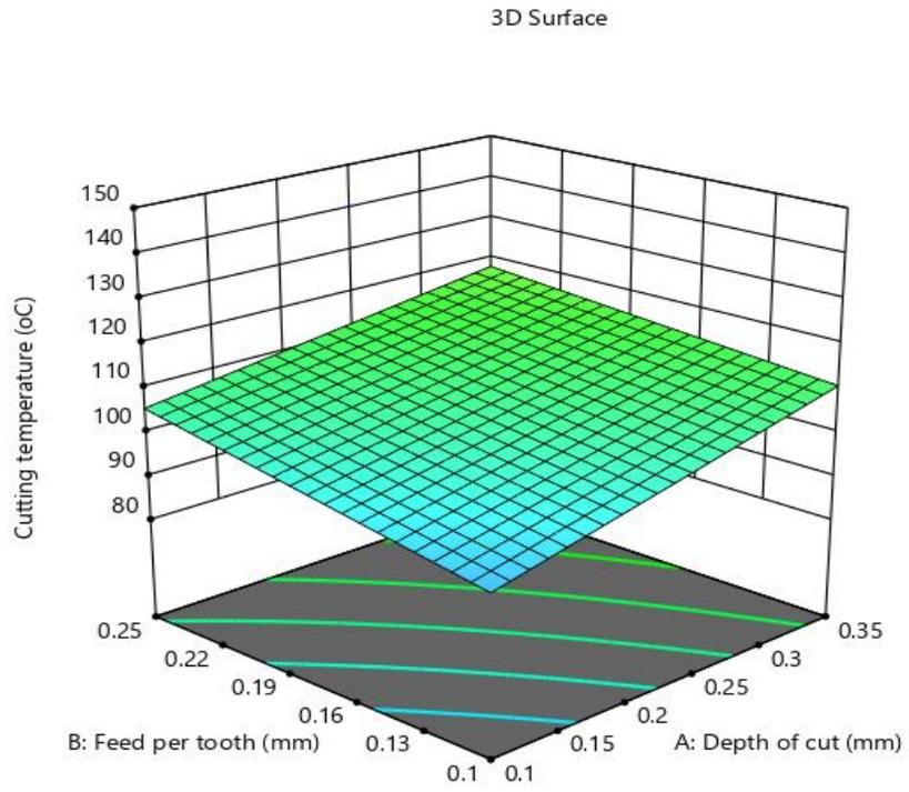
Fig. 4. Effect of DOC and FPT on cutting temperature
