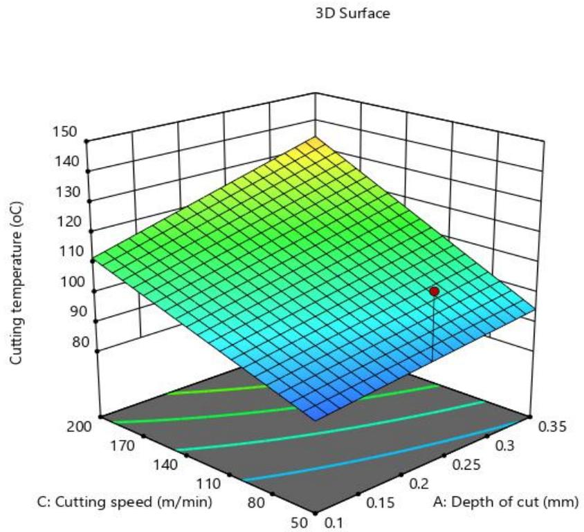
Fig. 5. Effect of FPT and CS on cutting temperature
