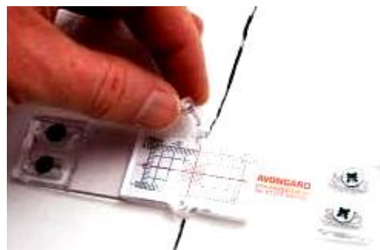
Figure 2. Installation of a mechanical cracker "Tell-Tale"
