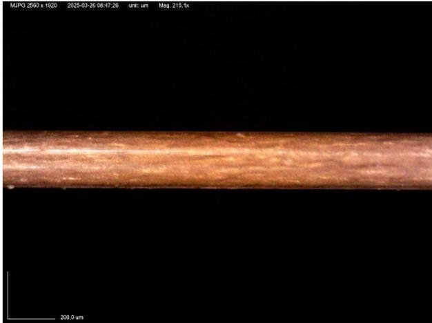
Fig. 8. Microscopic image of a new electrode (mag 215,1x).
