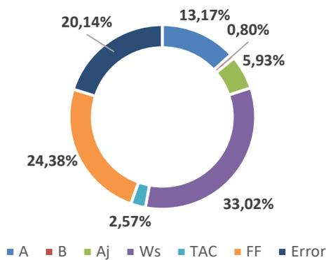
Fig. 5. The proportion of the influence of input parameters on electrode wear
