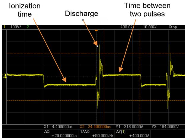
Fig. 2. The oscilloscope trace (the time between two pulses is set to 20  $\mu$ s in this case, which corresponds to the annotated time segment on the waveform –  $\Delta X = 20\mu$ s).
