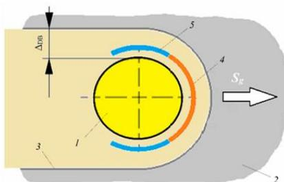
Fig. 3. Electrode wear at roughing, where (1) is a electrode, (2) workpiece, (3) machined surface, (4) front wear, (5) lateral wear [Grigoriev 2020]
