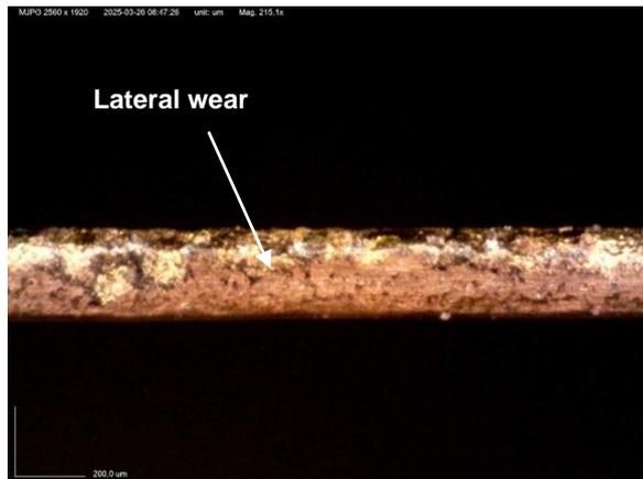
Fig. 9. Microscopic image of a wear electrode (mag 215,1x).
