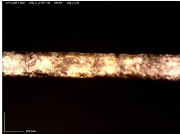
Fig. 10. Microscopic image of an electrode exhibiting predominant frontal wear (mag 215,1x).
