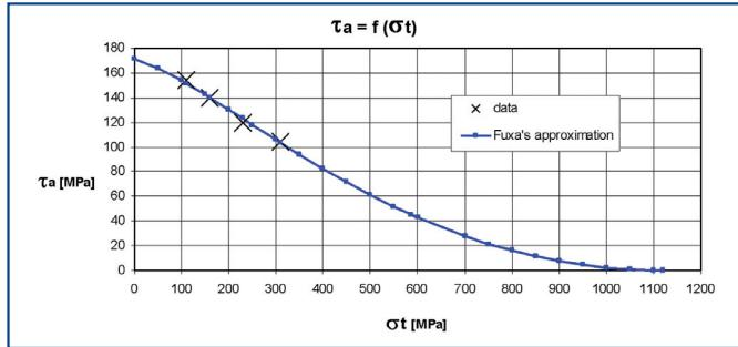
**Figure 3.** Influence of mean value tension stress for crack initialization
