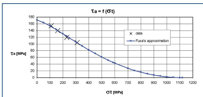
**Figure 4.** Fuxa's approximation for the combined loading
