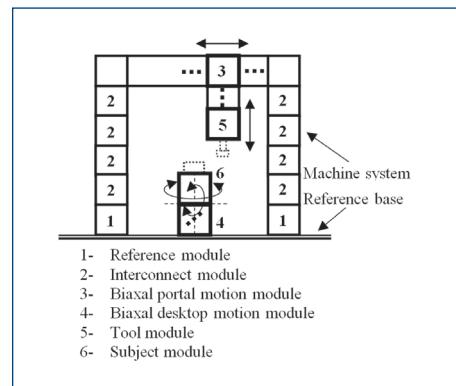
Figure 4. Reference assembly machine system
