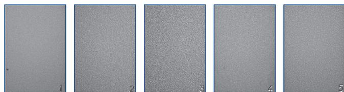
**Fig. 7.** Macrostructure of the steel S235 samples machined by 3-phase stream. Parameters: pressure=0.65 MPa; nozzle ID=8 mm; stand-off distance=150 mm; angle of attack  $\alpha=60^\circ$ . 1) SiO<sub>2</sub> 0.1 ÷ 0.4 mm; 2) SiO<sub>2</sub> 0.4 ÷ 0.8; 3) SiO<sub>2</sub> 0.8 ÷ 1.2; 4) Polgri 0.16 ÷ 0.5; 5) garnet #80
