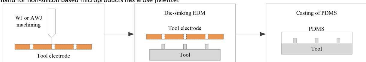
Figure 1. Microtooling process chain for casting of micromixer
