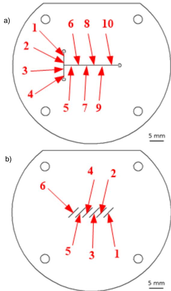
**Figure 3.** Contours of the tool electrodes used for tool insert machining by EDM. Measurement points are marked and numbered. a) Tool path for machining of the main channel – electrode A. b) Tool path for machining mixing elements in the main channel – electrode B.
