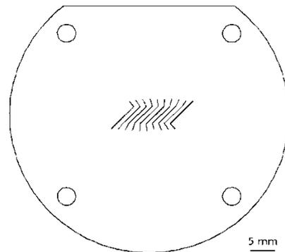
Figure 8. Tool path to machine tool electrode B with WJ machining.
