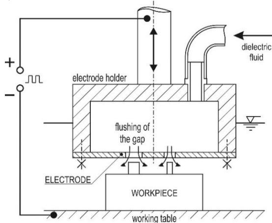
Figure 4. Electrode mounting while producing tool insert by die-sinking EDM.
