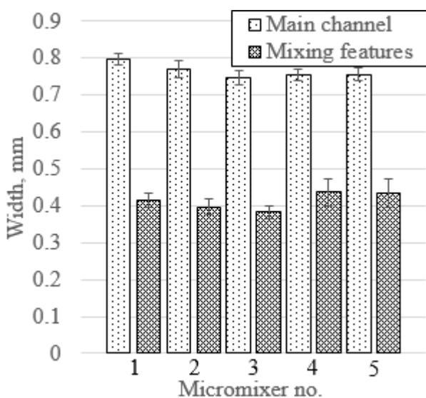
Figure 10. Dimensions obtained on five micromixers produced by casting.
