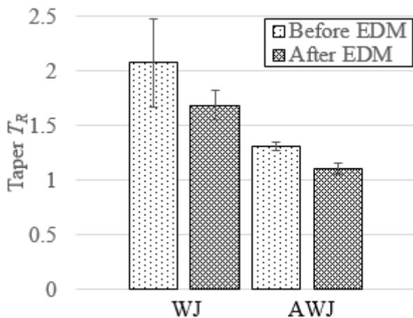
Figure 6. Taper on the electrodes measured before and after they were applied in EDM process
