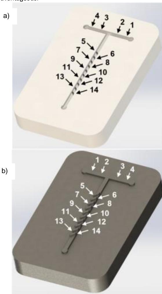
**Figure 2.** Tool insert with ribs used for casting of micromixer with grooves. Measurement points are marked and numbered. At points from 1 to 4, only the width of main channel was measured, at rest of the points both width of the main channel and width of the mixing features were measured.
