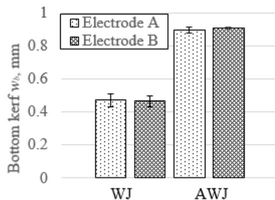
Figure 5. Kerf width measured on the bottom of the tool electrodes machined by WJ and AWJ technology. Electrode A is used to machine main channel channel whereas electrode B is used to machine mixing features in the channel.
