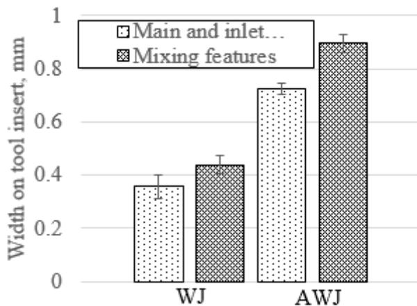
Figure 7. Measured widths of the features on the tool insert machined by EDM.
