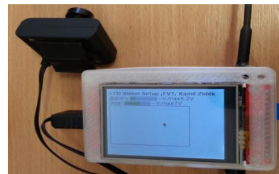
Figure 11. Embedded vision system used for image processing
