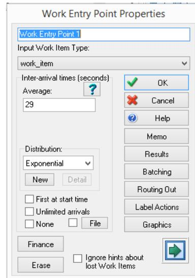
Figure 4. SIMUL8 Work Entry Point settings
