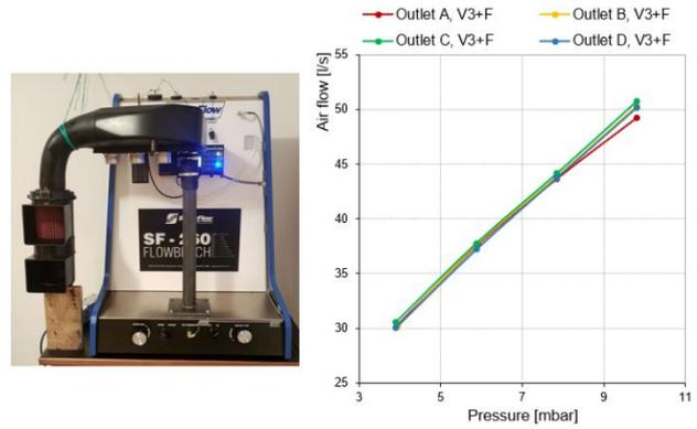
Figure 10. V3 airbox with the air filter measuring (left) and V3 airbox with the air filter flow characteristics (right)
