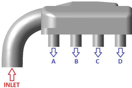
Figure 1. Airbox inlet and outlet openings
