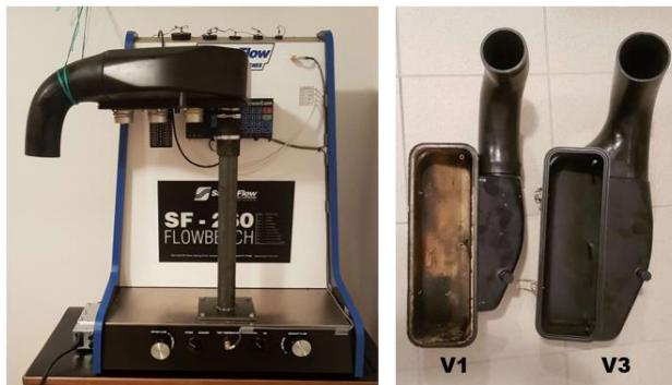
**Figure 7.** Measuring on the flow bench (left) and tested airbox variants (right)
