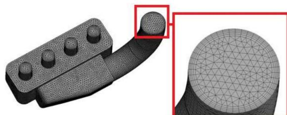
Figure 2. Numerical mesh on a serial airbox with a prismatic layer detail
