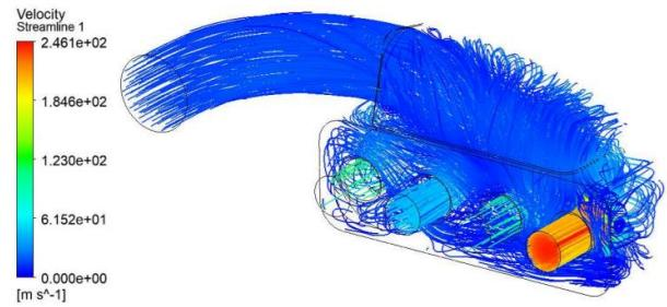
**Figure 5.** Air flow visualization during the D cylinder filling (airbox V1)
