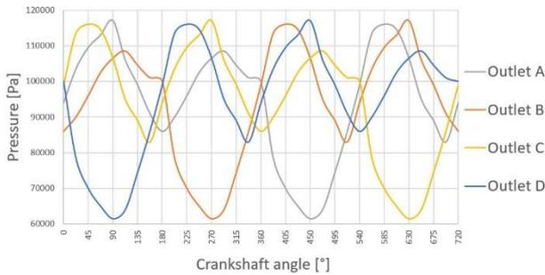
Figure 3. Pressure wave on individual outputs in one cycle
