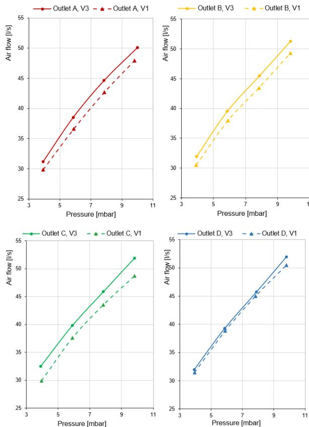
**Figure 9.** Flow characteristics of serial airbox (V1) and modified airbox (V3) - comparison of individual outputs
