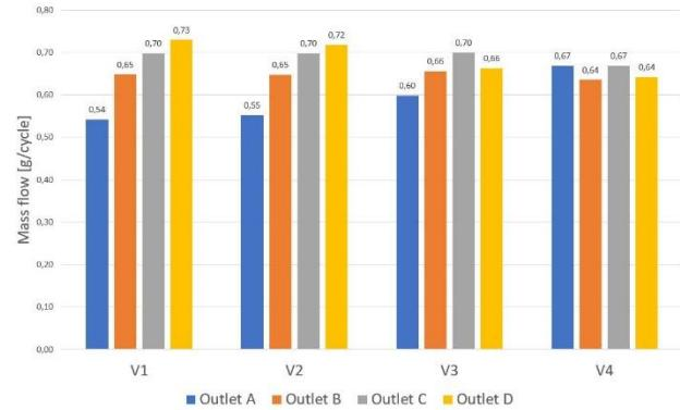
**Figure 6.** Comparison of mass flows through individual outlets during one suction cycle
