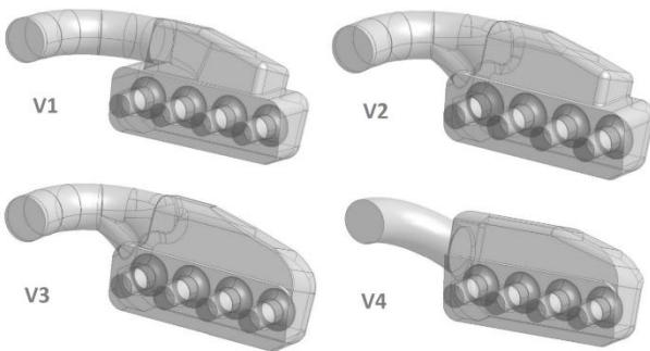
**Figure 4.** Airbox variants designed for CFD simulation
