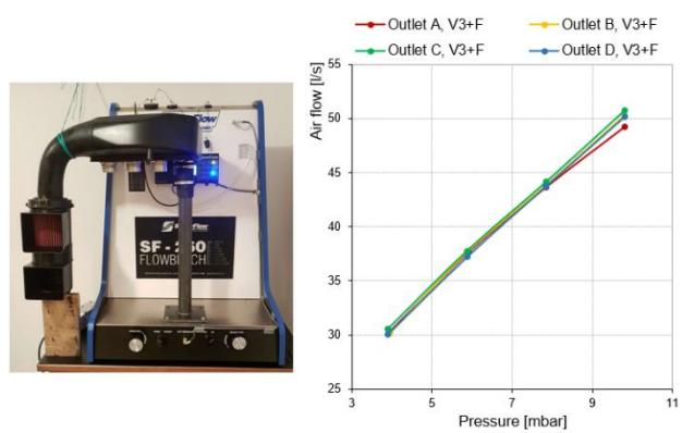
**Figure 10.** V3 airbox with the air filter measuring (left) and V3 airbox with the air filter flow characteristics (right)
