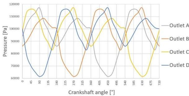
**Figure 3.** Pressure wave on individual outputs in one cycle
