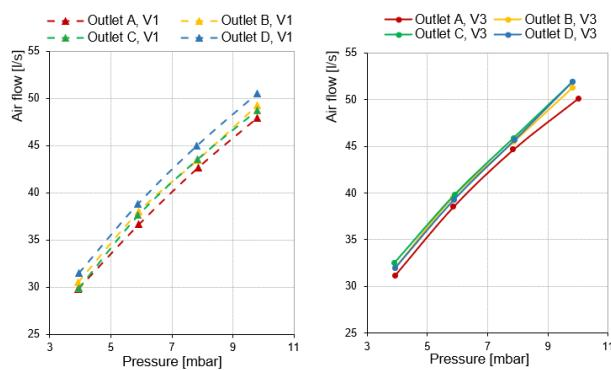
**Figure 8.** Flow characteristics of serial airbox (V1) and modified airbox (V3)
