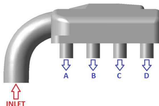
Figure 1. Airbox inlet and outlet openings
