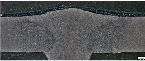
Figure 4. Macrostructure of the sample R-2.1A, the scale in the bottom right corner represents 2 mm
