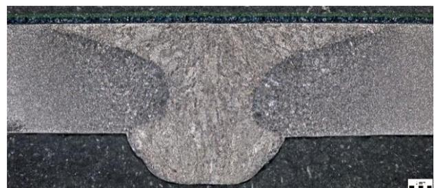
Figure 10. Macrostructure of the sample RB-2.4B, the scale in the bottom right corner represents 2 mm
