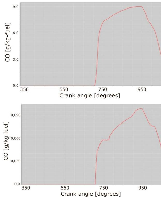
**Figure 5.** Evaluation of carbon monoxide (CO) emissions based on the crankshaft position (upper curve corresponds to the standard solution, lower curve pertains to the designed combustion chamber)
