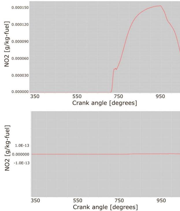
**Figure 4.** Examination of nitrogen oxide emissions in relation to the crankshaft position (upper curve for the standard solution, lower curve for the designed combustion chamber)
