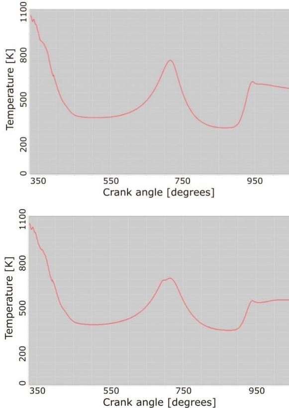
**Figure 3.** The variation of working temperature within the combustion chamber relative to the crankshaft position (upper curve represents the standard solution, lower curve indicates the specially designed combustion chamber).
