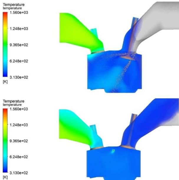
**Figure 2.** Examination of the working temperature in a combustion chamber with a standard piston (left); Investigation of the working temperature in a combustion chamber equipped with homogenization and controlled self-ignition of the fuel mixture using compression and a sparkplug (right)
