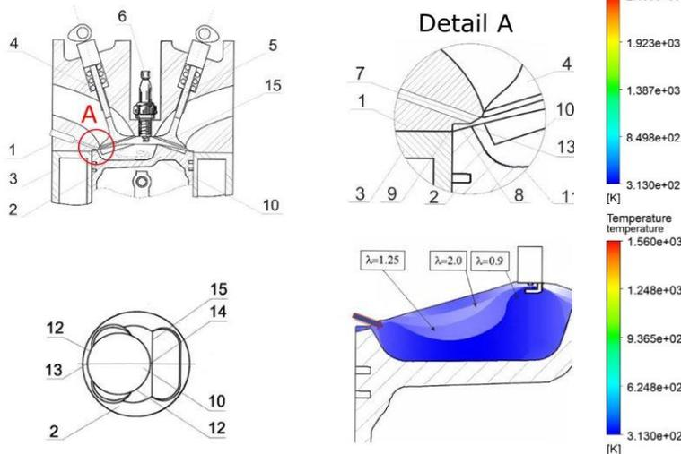
**Figure 1.** Combustion chamber incorporating homogenization and controlled compression-based self-ignition of the fuel mixture.
