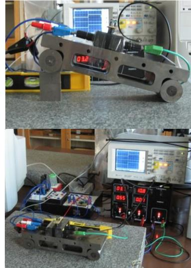
Figure 9. Calibration of tilt sensor.
