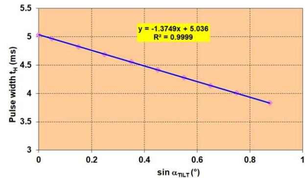
Figure 10. Static characteristic of the tilt sensor.
