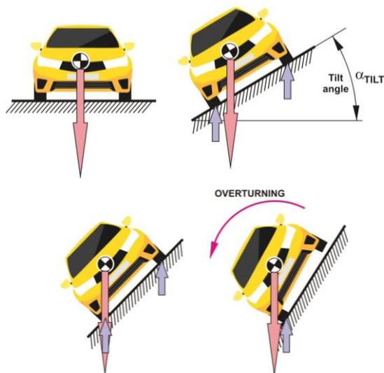
Figure 1. Measurement of tilt angle for detection of sideway vehicle instability
