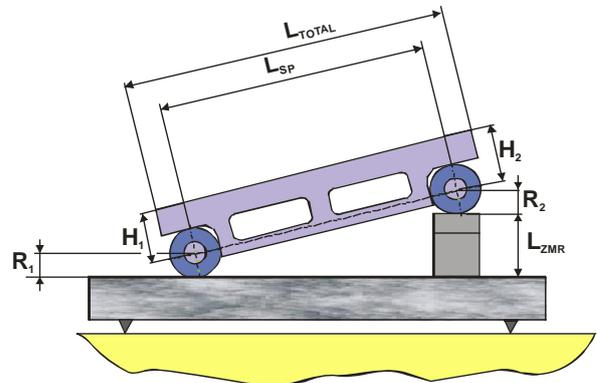
Figure 5. Dimensions measured using a coordinate measuring machine.
