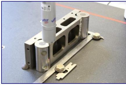
Figure 6. Measurement using a coordinate measuring machine.
