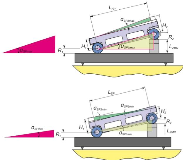
Figure 4. Model of the contact angle of the contact rollers with the horizontal plane  $\alpha_{SP1}$  (upper figure) and model of the angle of the upper surface of the body of the sine plate  $\alpha_{SP2}$  (lower figure).
