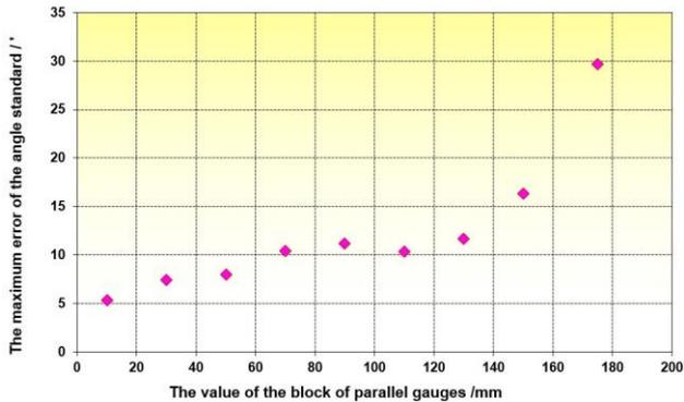
Figure 8. The maximum error of the tilt angle etalon at different values of the block of parallel gauges (or tilt angles) when considering the most unfavourable deviations of individual members of the tilt angle etalon.
