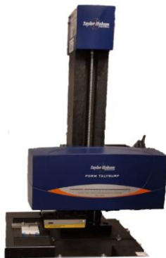
Figure 2. Measurement of the test sample using Form Talysurf PGI 1230
