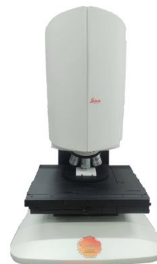
Figure 3. Sample measurement using a LEICA DCM8 microscope.
