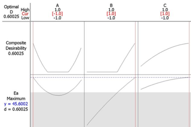
Figure 6. The optimal operational parameters chart of the crash box design for maximum EA
