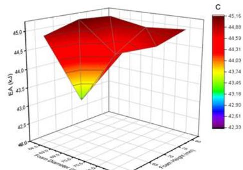
Figure 2. The effects of foam diameter and foam height on the EA
