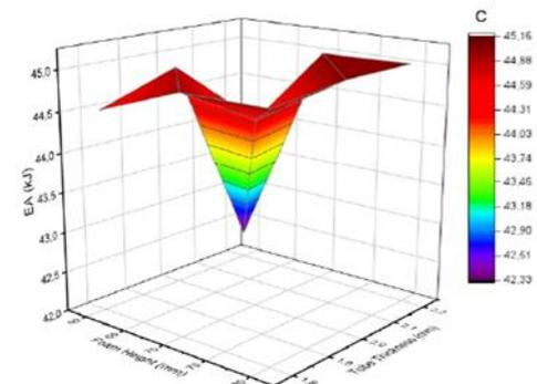
Figure 3. The effects of foam diameter and tube thickness on the EA
