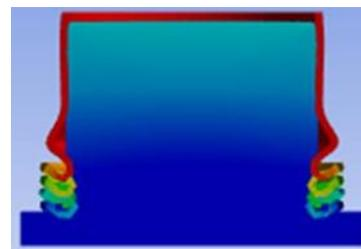
Figure 7. Deformation pattern results on the optimum design
