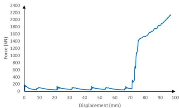
Figure 8. Load-Displacement curve on the optimum design crash box model
