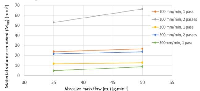
Figure 7. Graph of Material volume removed  $M_{VR}$  vs Abrasive mass flow  $m_a$
