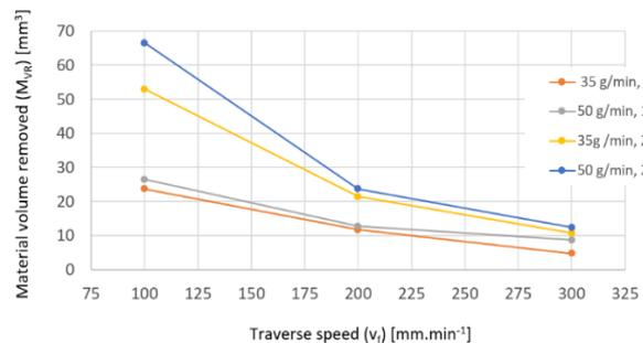
Figure 6. Graph of Material volume removed ( $M_{VR}$ ) vs traverse speed ( $v_f$ )
