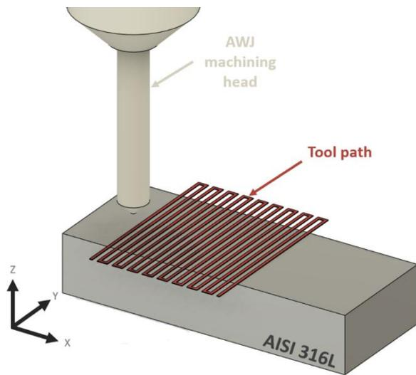
Figure 1. Schematic representation of machining during the experiment
