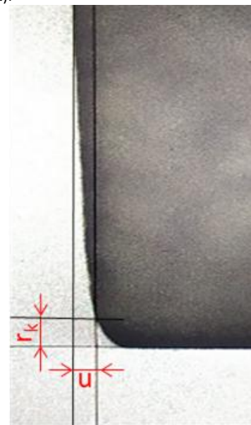
Figure 2. Measurement of perpendicularity or angularity tolerance u [mm] and edge radius r_k [mm] parameter
