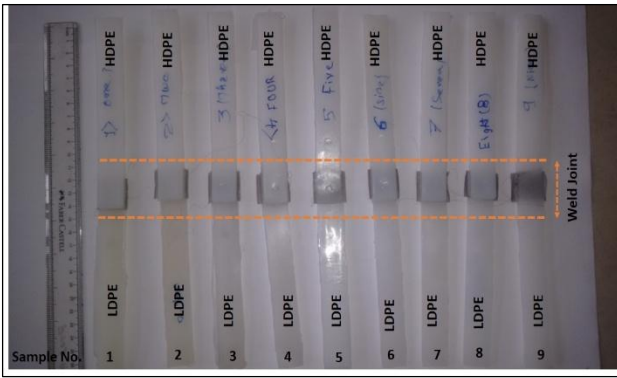
Figure 2. Various resistance welded joints at different experiment trials
