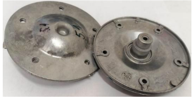
Figure 5. Electric motor flange cast
