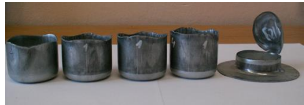
Fig. 9: View of drawn parts after drawing test from blanks with diameters 120, 121, 123, 127 and 129 mm.
