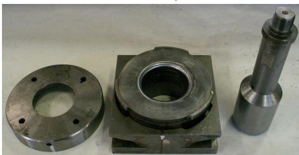
Fig. 8: View of a drawing tool used for determination of limiting drawing ratio according to Schmidt.
