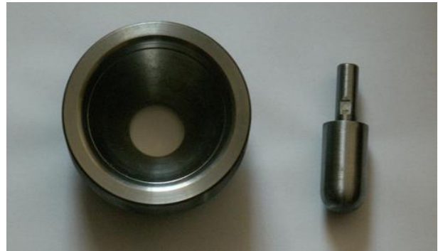
Fig. 4: Drawing die used for the Fukui cup test.
