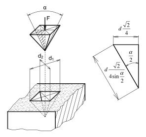
Figure 3. Scheme of Vickers hardness measurement
