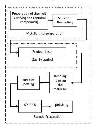
Figure 2. Scheme of samples preparing for the micro hardness measurement
