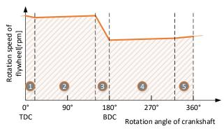
**Figure4.**Rotation speed of countershaft (significant phase of stroke)
