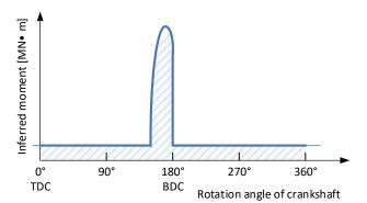
Figure2. Typical torque of crank shaft during work stroke
