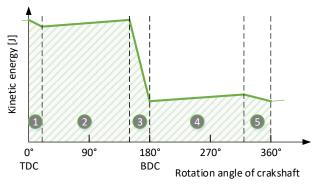
Figure3. Energy accumulated in moving parts of crank press (significant phase of stroke)
