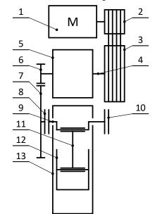
Figure 1.Diagram of typical crank forging press drive (1 – Electric motor; 2 – Drive pulley of motor; 3 – Drive pulley of countershaft; 4 -Countershaft; 5 -. Flywheel; 6 – Pinion of countershaft; 7 – Gear wheel of clutch; 8 - Clutch; 9 – Crank shaft; 10 - Brake; 11 – Connecting rod; 12 - Ram; 13 – Press frame)
