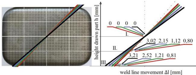
**Figure 7.** Weld movement on the bottom of diagonally welded blank
