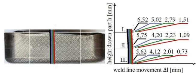
**Figure 4.** Weld movement on the wall of transversely welded blank
