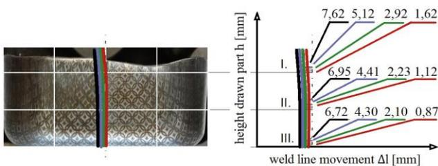
**Figure 2.** Weld movement on the wall of longitudinally welded blank
