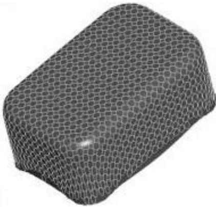
**Figure 1.** Experimental drawn part with a deformation grid of round elements
