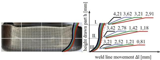
**Figure 6.** Weld movement on the wall of diagonally welded blank
