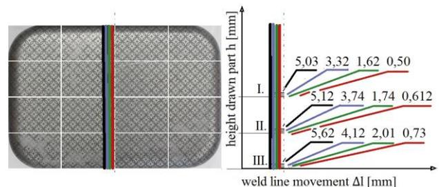
**Figure 5.** Weld movement on the bottom of transversely welded blank
