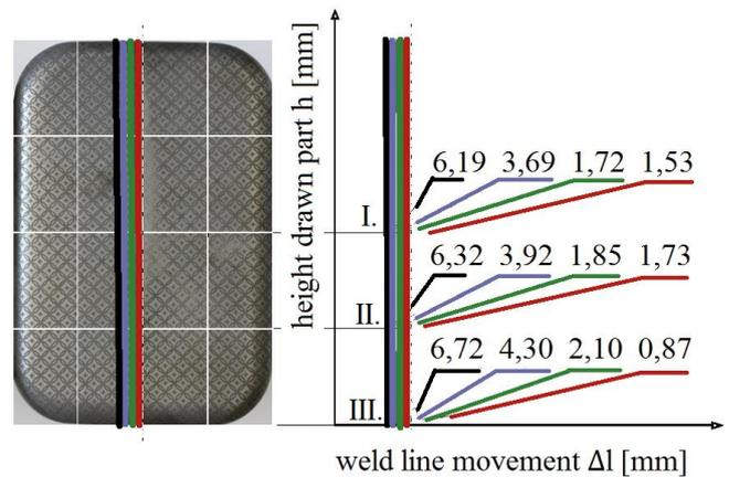
**Figure 3.** Weld movement on the bottom of longitudinally welded blank
