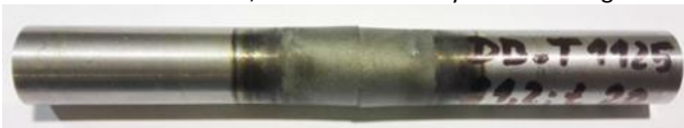
Figure 5. Diffusion jointed sample at temperature 1125°C; holding force 1.2 kN and exposure time 1200 sec
