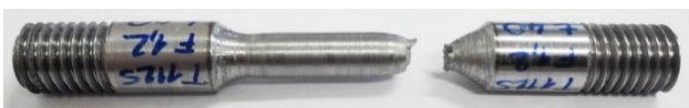
Figure 6. Diffusion jointed samples after static tensile test revealed fracture beyond the diffusion joint area
