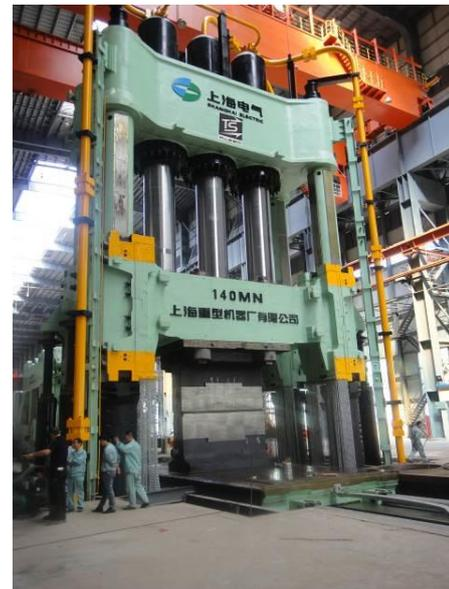
Figure 7. Assembled CKV 120/140 press ready for testing
