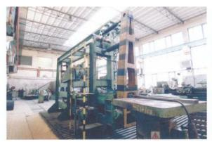
Figure 2. Fatigue machine P5-GIG3 [Zrnik 2000, Tomkova 2001]
