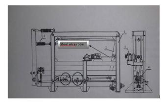
Figure 1. Fatigue machine P5-GIG3 1-Steel frame, 2-arm, 3-springs, 4-wheelchair, 5-drive [Zrnik 2000, Tomkova 2001]
