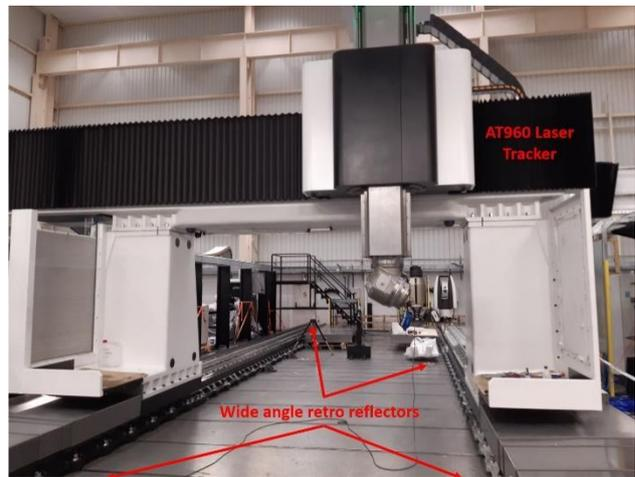
Fig. 8: Real integration exercise within the ZAYER THERA machine tool with a LEICA AT960 laser tracker.
