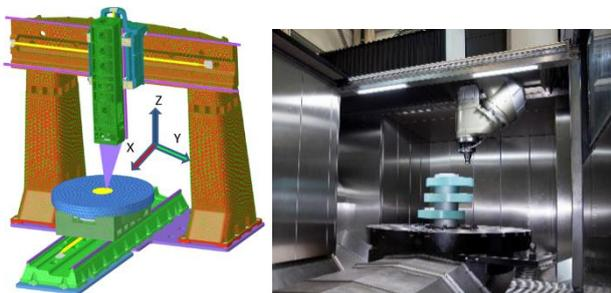
Fig. 4 a) the ZAYER ARION G MT FEM Model and b) the MT at Tekniker facilities.
