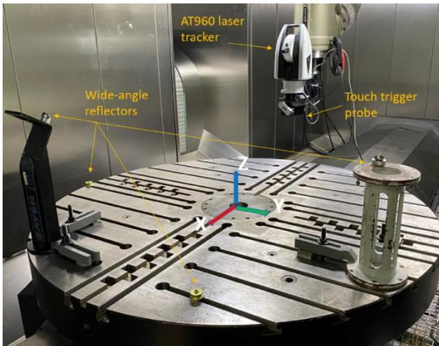
Fig. 7: Real integration exercise within the ARION G machine tool with a LEICA AT960 laser tracker.
