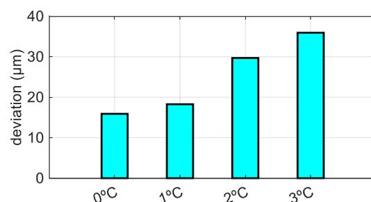
Fig. 6 Influence of fiducial point thermal drift on MIIM expanded measurement uncertainty.
