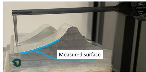
Figure 4. Roughness measurement on the test workpiece
