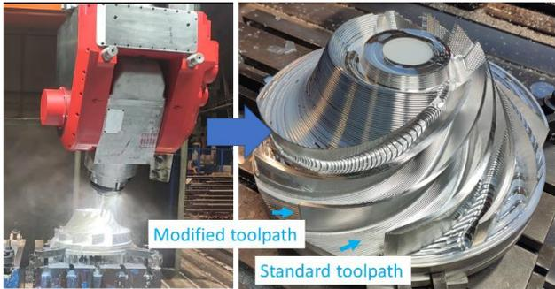
Figure 7. Machining of turbine hubs on the FRF machine tool
