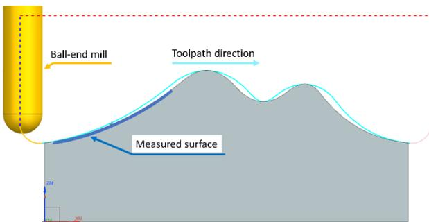
Figure 3. Test workpiece with toolpath set
