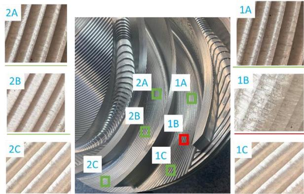
Figure 9 Optical quality of the measured areas on the turbine hub
