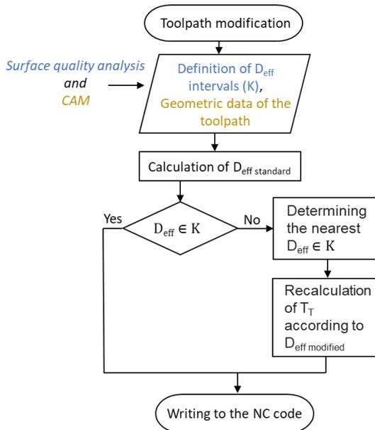
Figure 2. Toolpath modification scheme
