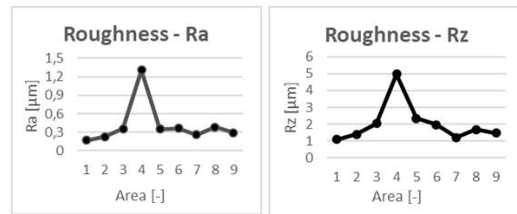
Figure 5. Measured surface roughness in the direction of ball-end mill toolpath
