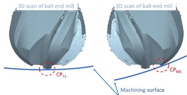
Figure 6. definition of two areas with deteriorated surface quality
