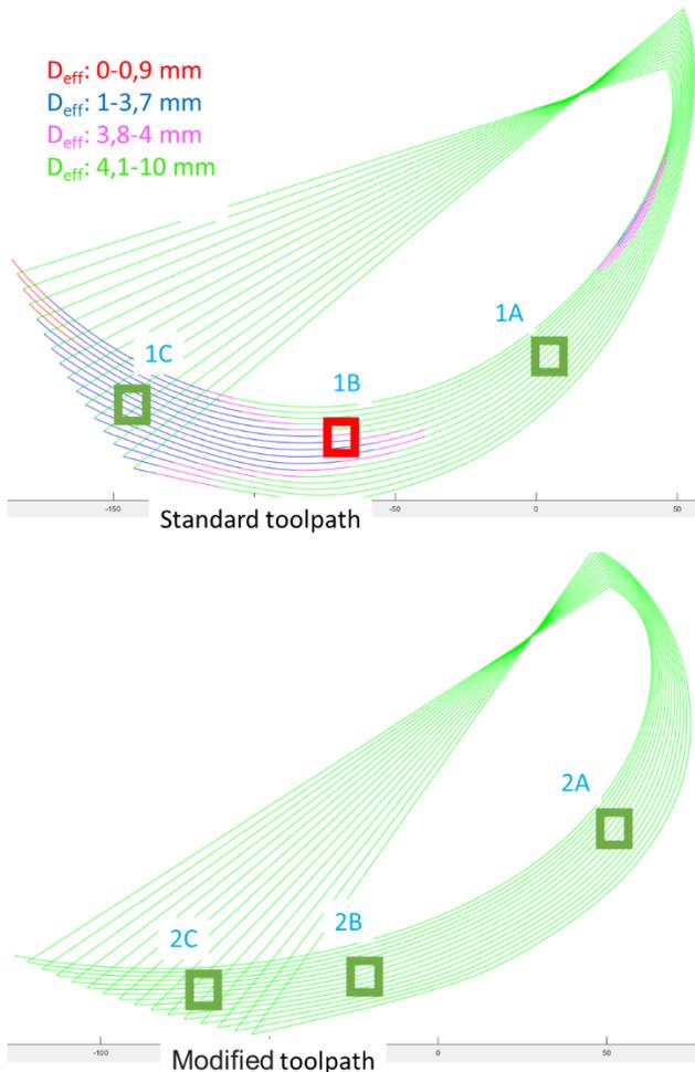
Figure 8. Visualization of areas on the hub toolpath with the risk of workpiece quality deterioration
