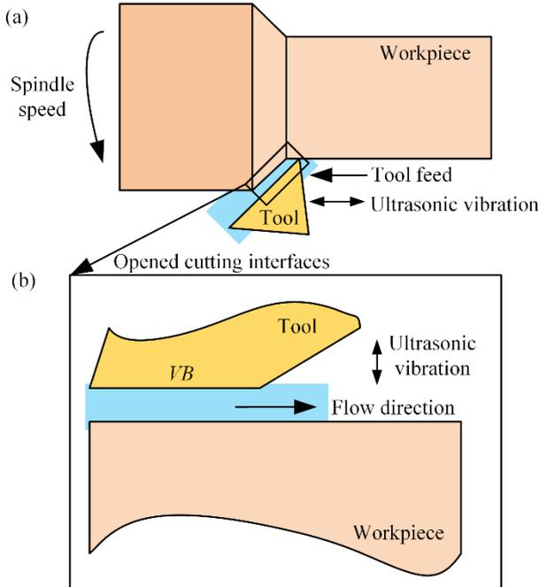
Fig. 1: Schematics of (a) HUVIC process and (b) cutting interfaces.
