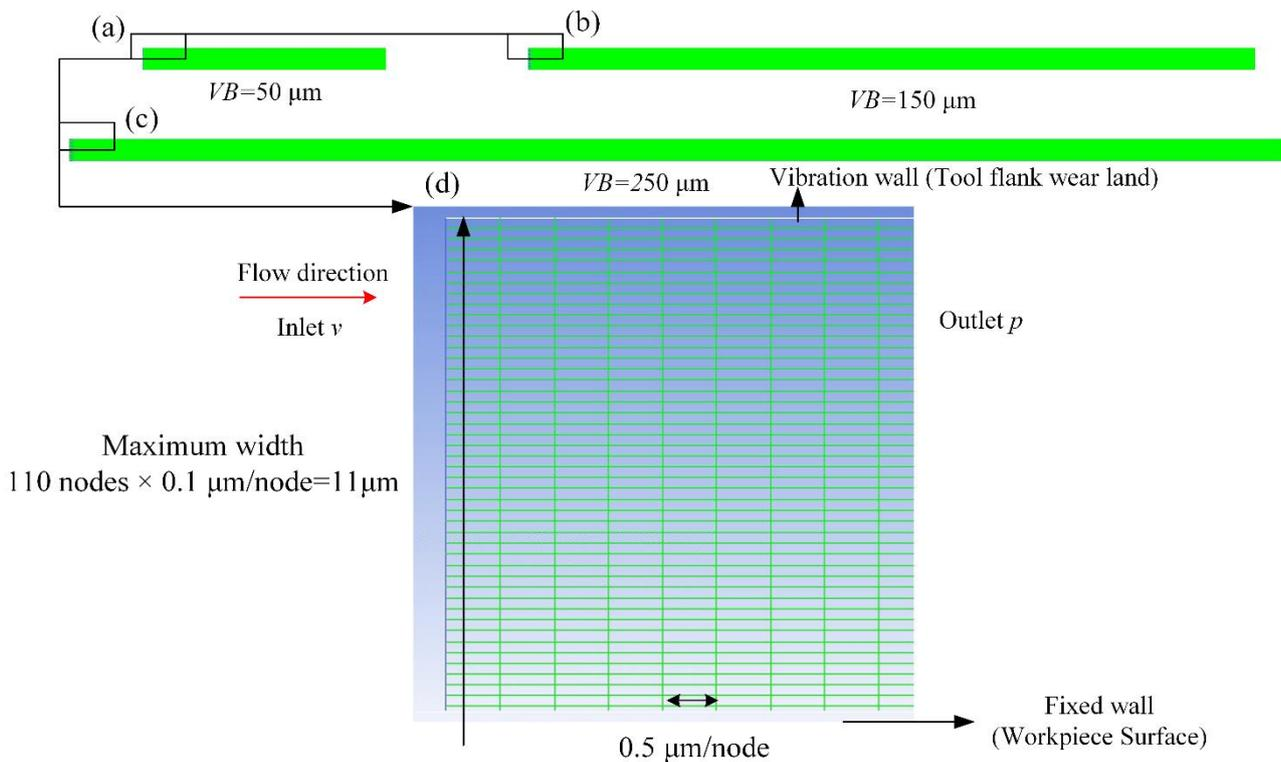
Fig. 3: Mesh grids of CFD set up. (a)  $VB=0.05$  mm, (b)  $VB=0.15$ , (c)  $VB=0.25$  and (d) detailed information
