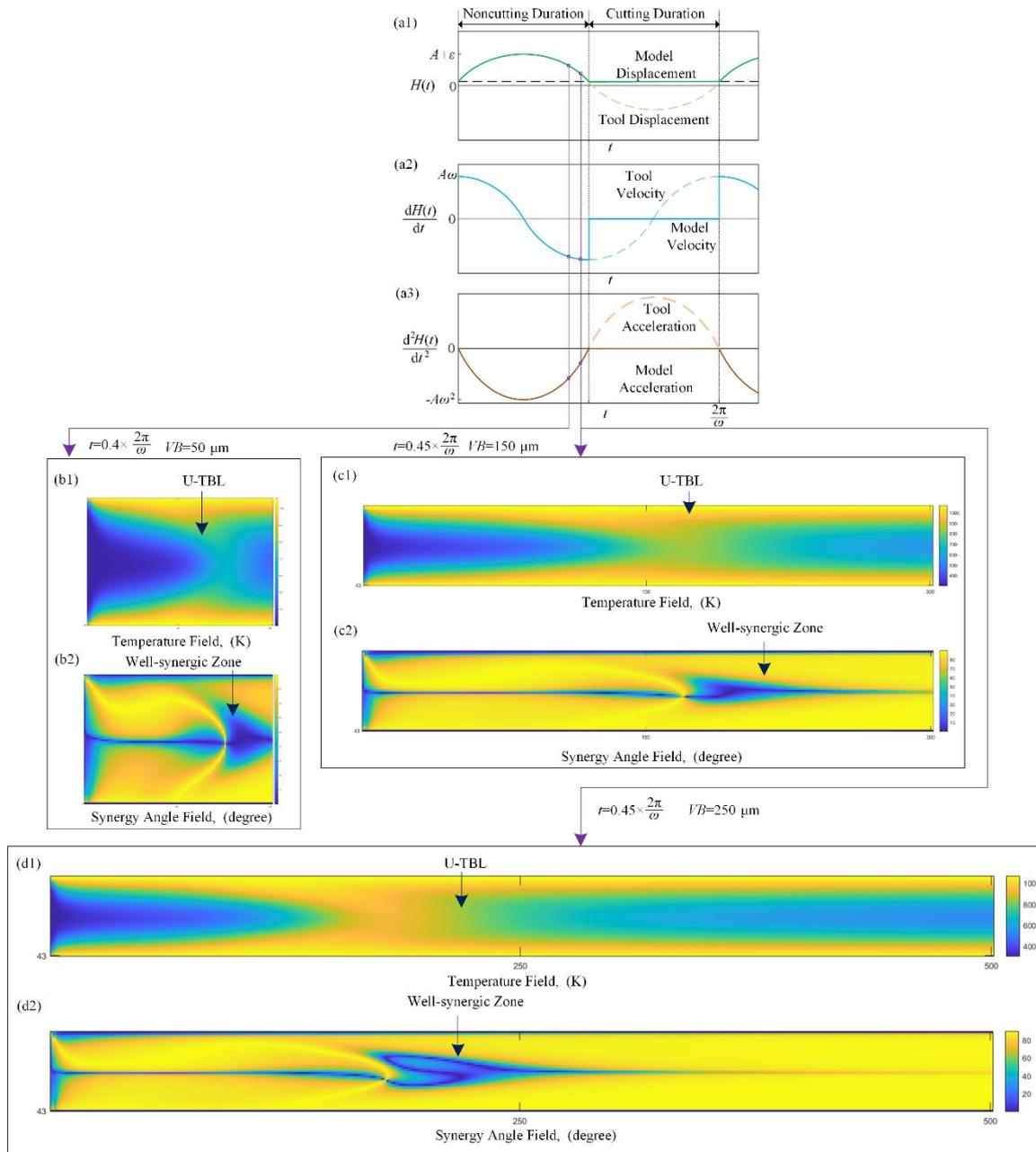
Fig. 6: CFD results of 1 m/s inlet velocity, (a) dynamic mesh boundary wall, 1, displacement, 2, vibration velocity, 3, vibration acceleration. selected moments of U-TBL disappearance of (b)  $VB=0.05$  mm, (c)  $VB=0.15$  mm and (d)  $VB=0.25$  mm. 1 and 2 are temperature and synergy angle fields, respectively.
