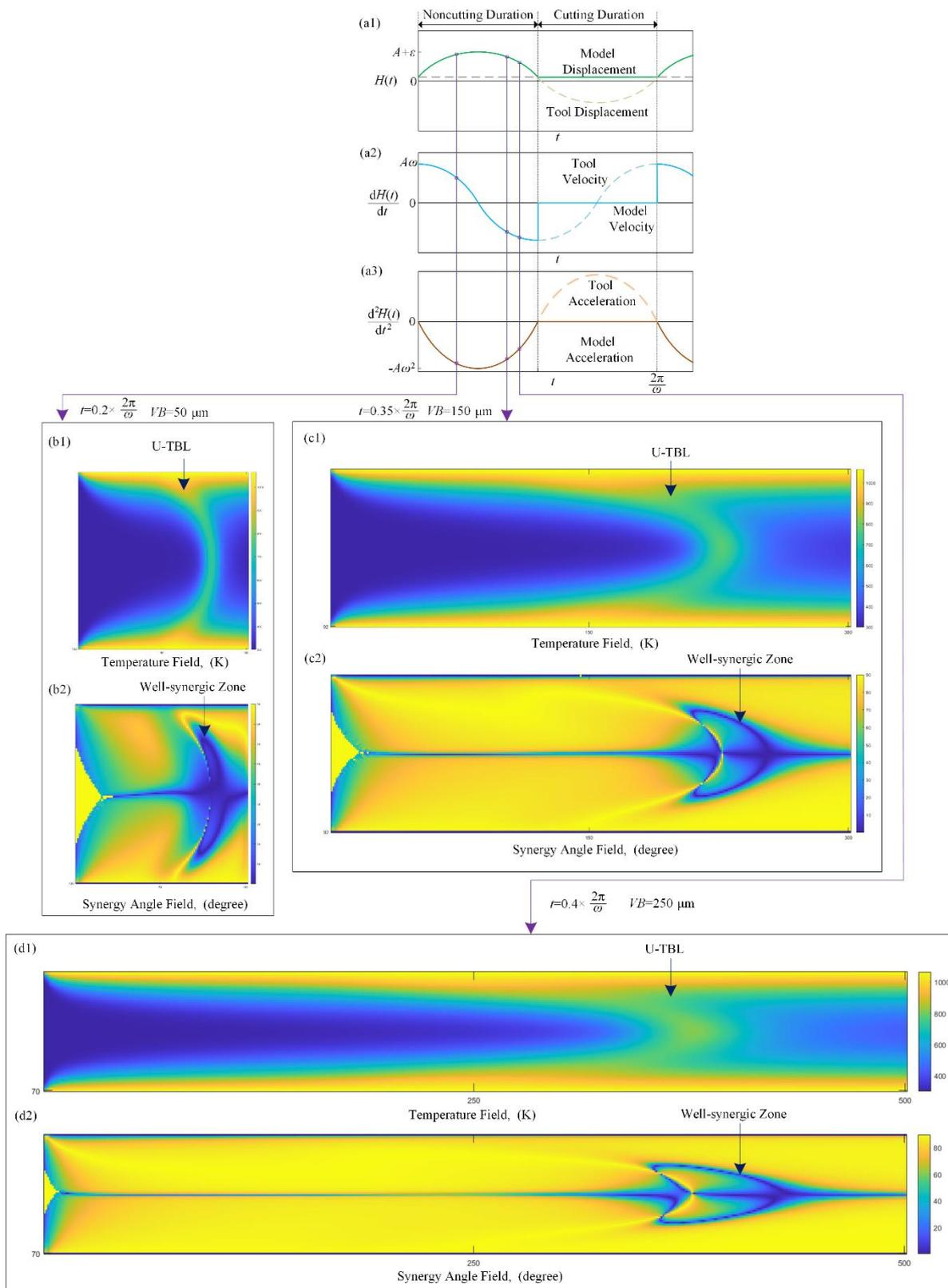
Fig. 7: CFD results of 5 m/s inlet velocity, (a) dynamic mesh boundary wall, 1, displacement, 2, vibration velocity, 3, vibration acceleration. selected moments of U-TBL disappearance of (b)  $VB=0.05 \text{ mm}$ , (c)  $VB=0.15 \text{ mm}$  and (d)  $VB=0.25 \text{ mm}$ . 1 and 2 are temperature and synergy angle fields, respectively.
