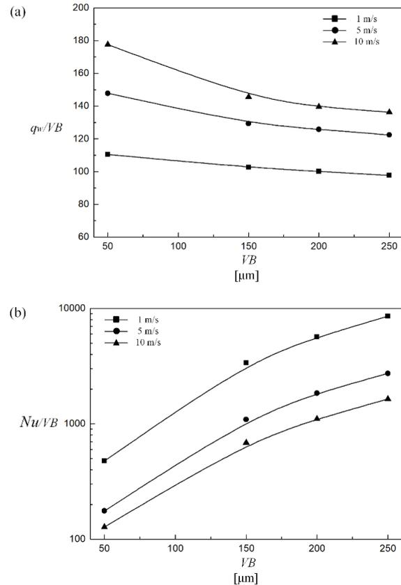
Fig. 5: (a) heat flux and (b) Nusselt Number per unit characteristic length within cutting interfaces of different length flank wear  $VB$  at cutting speeds of 1, 5 and 10 m/s, respectively. Data of  $VB=0.2$  mm was cited and modified from [Zhang 2023].
