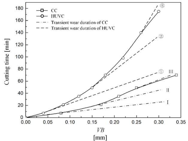
Fig. 2: Tool wear progress modified from Lu 2020.
