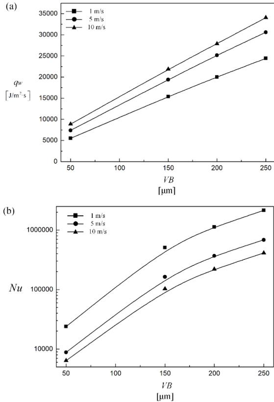
Fig. 4: (a) heat flux and (b) Nusselt Number within cutting interfaces of different flank wear  $VB$  at cutting speeds of 1, 5 and 10 m/s, respectively. Data of  $VB=0.2$  mm was cited and modified from [Zhang 2023].
