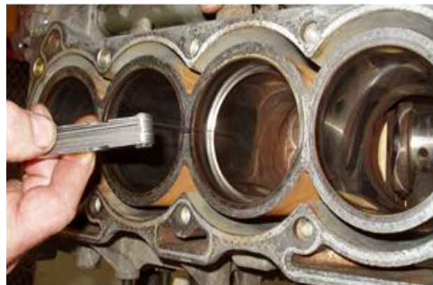
Figure 3. Measurement of piston ring locks clearance in a cylinder
