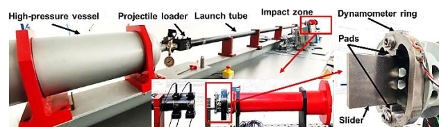
Fig. 2. Slider-on-pads tribometer configuration.
