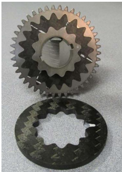
Figure 9. Prototype hybrid spur gear
