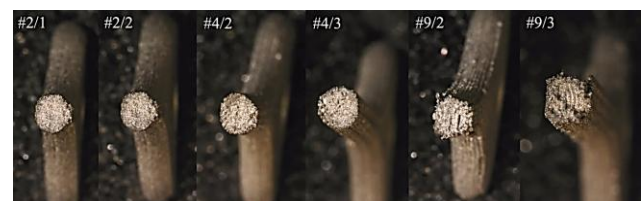
Figure 10. Fracture surfaces of tensile specimens with layer heights of 0.2, 0.3, and 0.4 mm (left to right), showing rougher texture and weaker interlayer bonding with increasing layer height.
