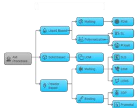
Figure 1. Classification of Additive Manufacturing Processes based on energy source, and deposition technique
