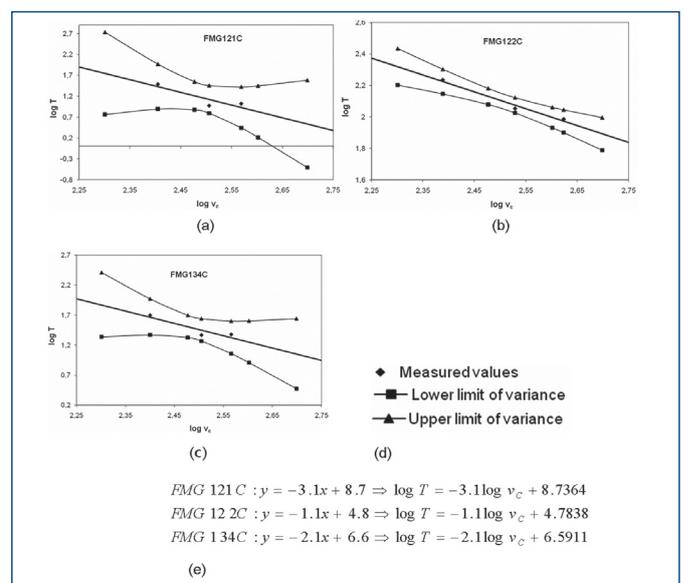
Figure 4. Graphic dependence of  $\log T$  values plotted against the  $\log v_C$  values for all three CTI, (a to c); including symbols (d) and corresponding Equations (e).
