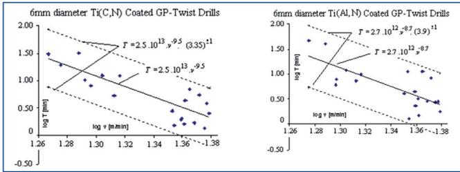
**Figure 2.** An example of empirical Taylor-type relationship between drill life and cutting speed for the uncoated (a), TiN coated (b), Ti(C, N) coated (c) and Ti(Al, N) coated (d), drills, adopted from source [Audy 2007].
