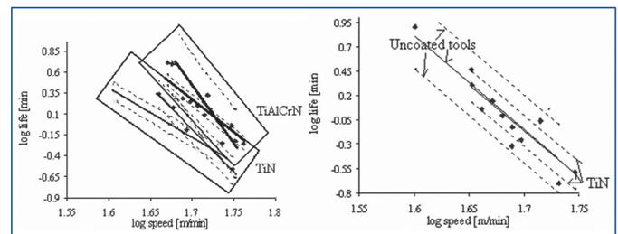
Figure 1. Effects of composition of (Ti,Al,Cr)N and TiN coatings, left, and TiN coated and uncoated drills when dry drilling grey cast iron. [Audy et al 2002], and [Audy 2009] when dry drilling grey cast iron.
