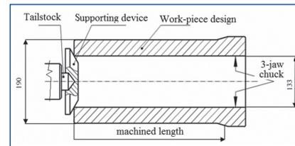
**Figure 3.** A sketch showing the actual design of experimental work-piece material, after source [Kovalčík 2008].
