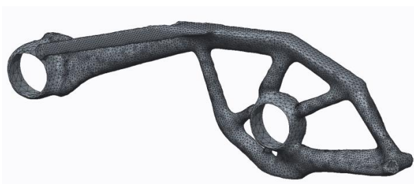
Figure 9. Type B rocker, m=0.104 kg, average element size 1.5 mm
