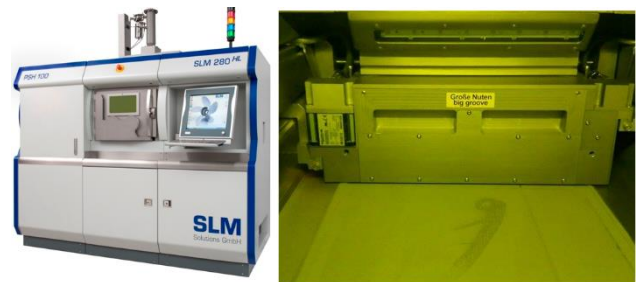
Figure 17. SLM 280 HL machine with a view to the workspace.
