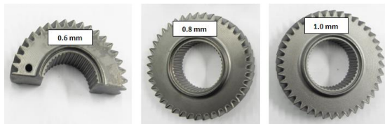
Figure 4. The carburizing gear wheels of steel by CSN 14020
