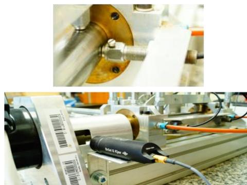
Figure 2. Proximity sensors and a rotational speed sensor
