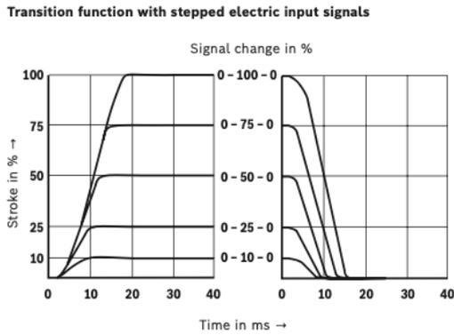
Figure 1. Typical step responses of the valve opening for different magnitude of the input step signals [Bosch Rexroth AG 2019]
