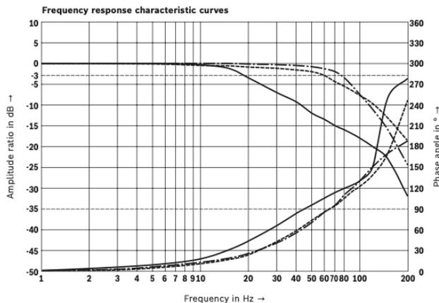
Figure 2. Typical Bode plots of the servovalve for different magnitudes of the input signals [Bosch Rexroth AG 2019]
