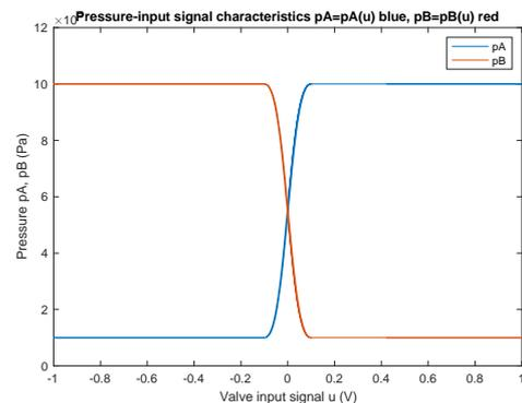
**Figure 7.** Simulated pressure characteristics  $p_A=p_A(u)$  and  $p_B=p_B(u)$
