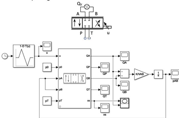
**Figure 4.** Simulation model for the measurement of the flow-input signal characteristics and corresponding hydraulic circuit
