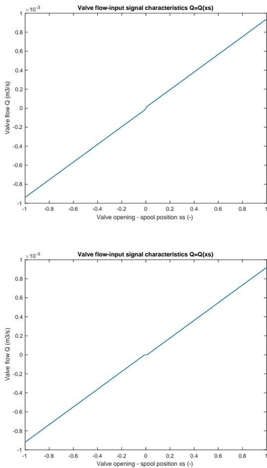
**Figure 5.** Simulated flow characteristics for negative (upper graph) and positive (lower graph) overlap
