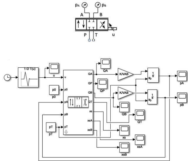
**Figure 6.** Simulation model for the measurement of the pressure – input signal characteristic  $p_A=p_A(u)$ , resp.  $p_B=p_B(u)$
