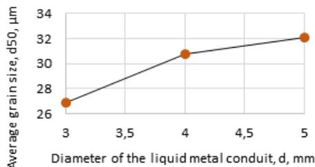
**Figure 8.** Average particle size dependence on liquid metal conduit diameter
