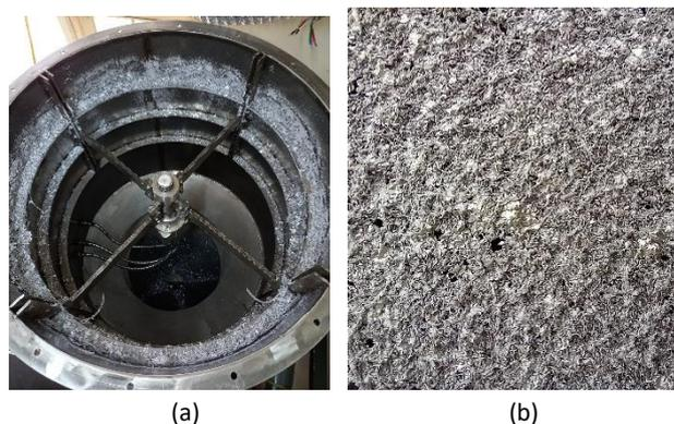
**Figure 11.** The phenomenon of metal adhesion and accumulation on the wall of the dispersion chamber ( $h = 3$  cm)
