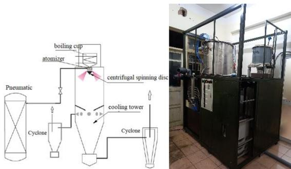
**Figure 3.** Technological diagram (left) and actual image (right) of metal 3D printing powder fabrication equipment.
