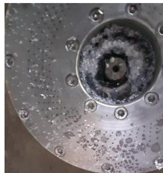
**Figure 10.** Accumulation of liquid metal at the dispersed gas ring and heating copper tube ( $h = 1$  cm)
