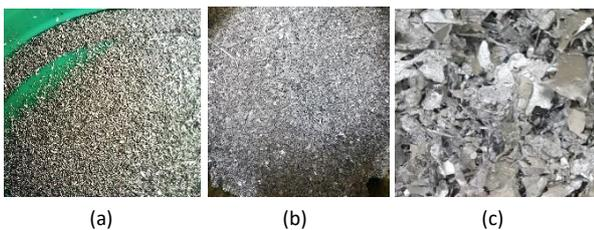
**Figure 5.** Images of products of AlSi10Mg liquid alloy dispersion
