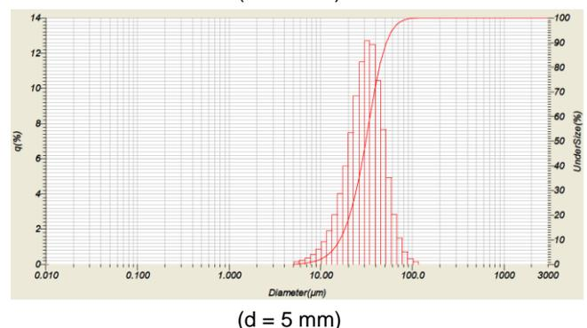
**Figure 7.** Results of determination of particle size distribution of metal powder group with particle size less than 100  $\mu\text{m}$
