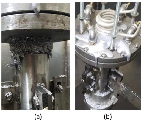
**Figure 9.** Accumulation of liquid metal at the dispersion gas ring (with  $h = 0,5$  cm)
