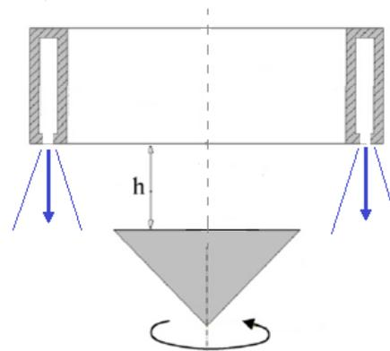
Figure 2. Illustration of geometrical parameters of metal powder fab equipment
