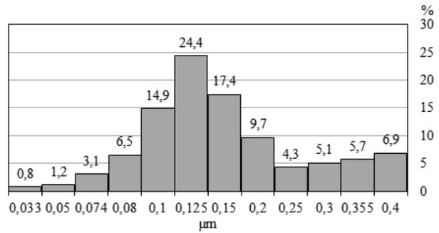
**Figure 6.** Particle size distribution of metal powder with a size less than 0.4 mm
