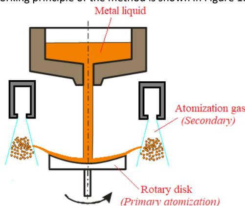
Figure 1. Diagram of dispersion of molten alloy using centrifugation and high-pressure inert gas
