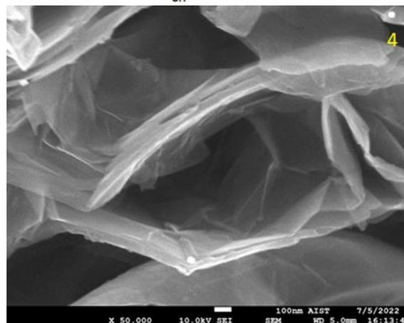
Figure 2. Multilayer graphite oxide
