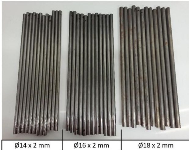
Figure 3. Measured cold-drawn seamless precision steel tubes: 36 specimens (500 mm in length), obtained by cutting three 6 m tubes into three groups of 12 pieces: OD \varnothing 14 mm, \varnothing 16 mm and \varnothing 18 mm (all with WT of 2 mm)
