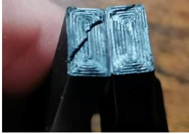
Figure 11. Fracture surface of the test specimen printed at print speed of 50 mm/s and nozzle temperature of 230 °C [Kruzliak 2024]
