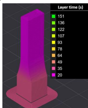
Figure 3. Illustration of the layer time parameter in the gauge section of the test specimen, where t_v = 3.1 s [Kruzliak 2024]
