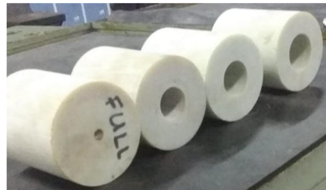
Figure 2. Fiberglass filler specimens: solid (0 mm) and with central holes of 24 mm, 28 mm, and 32 mm diameter
