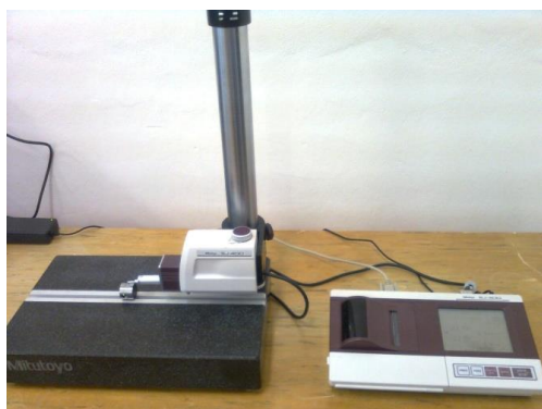
Figure 2. Profilometer MiruoyoSurfTest SJ400
