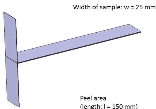
Figure 1. Geometry of the sample for the T-peel test
