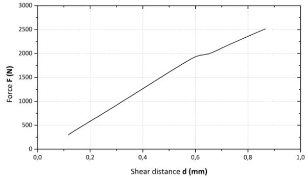
Figure 9. Force  $F$  (N) vs. shear distance  $d$  (mm) for the lap shear test
