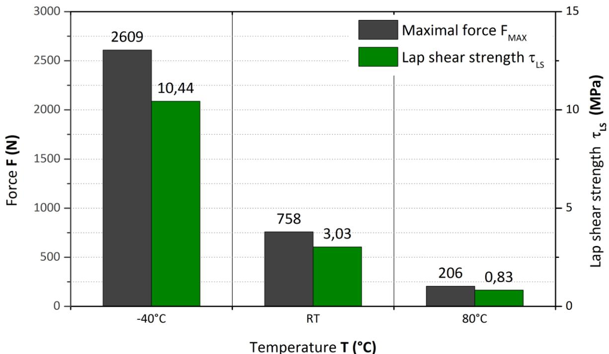
Figure 10. Major results from the lap shear test:  $F_{MAX}$  and  $\tau_{LS}$  in dependence on the testing temperature
