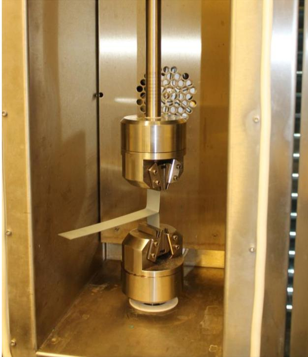
Figure 3. The T-peel test – arrangement of the experiment
