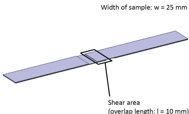
Figure 2. Geometry of the sample for the lap shear test
