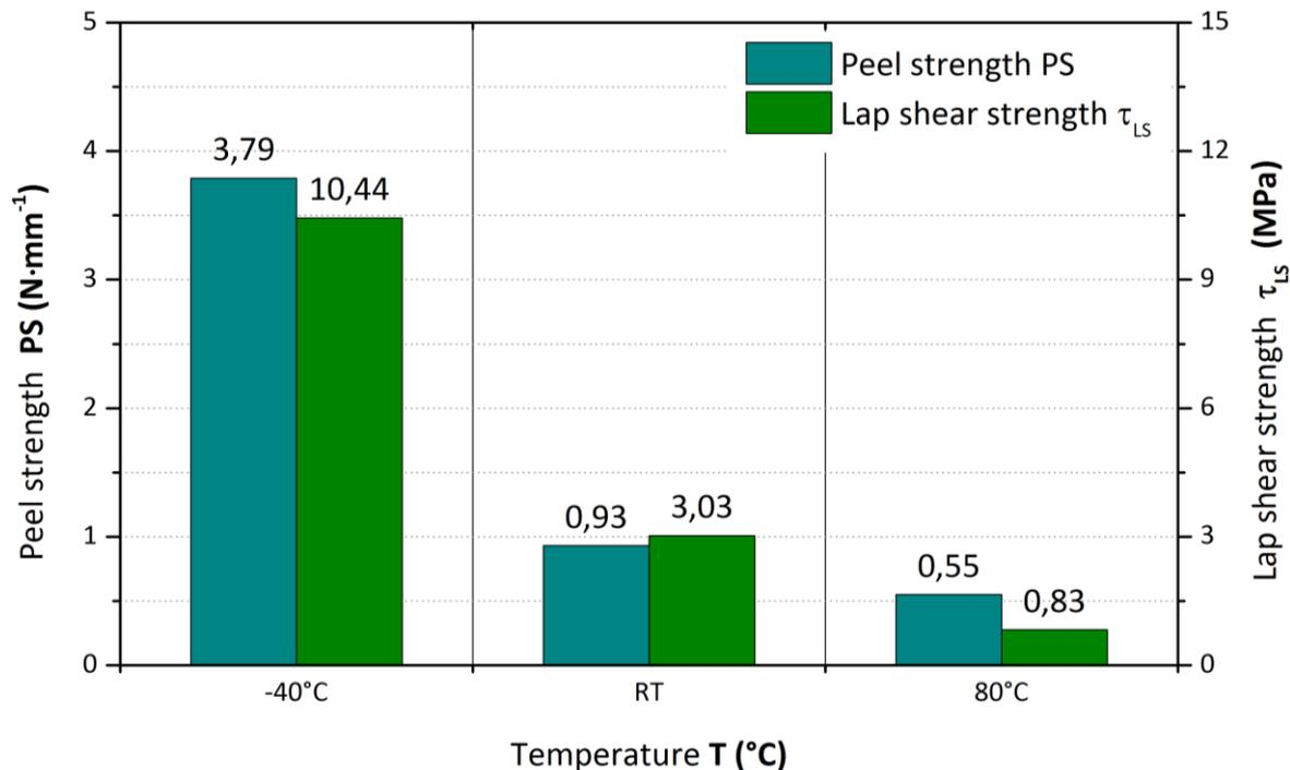
Figure 11. Comparison of the PS and  $\tau_{LS}$  in dependence on the testing temperature
