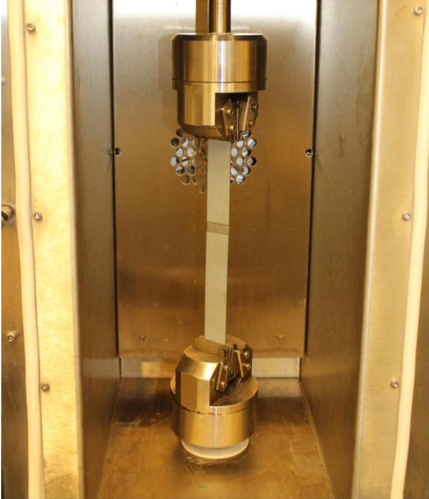
Figure 8. The lap shear test – arrangement of the experiment
