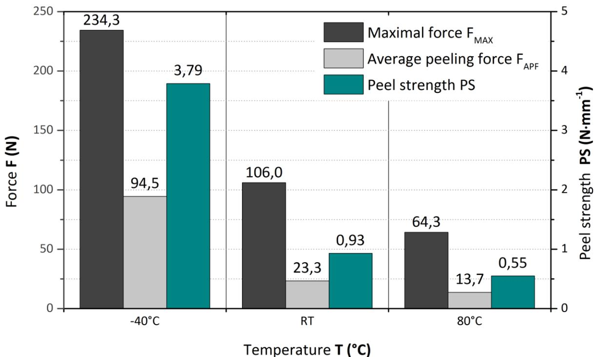
Figure 7. Major results from the T-peel test:  $F_{MAX}$ ,  $F_{APF}$  and PS in dependence on the testing temperature
