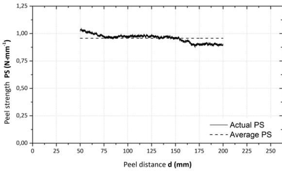
Figure 5. Computation of the peel strength PS ( $N \cdot mm^{-1}$ ) – 1<sup>st</sup> approach
