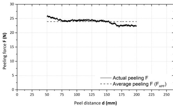
Figure 6. Computation of the peel strength PS ( $N \cdot mm^{-1}$ ) – 2<sup>nd</sup> approach
