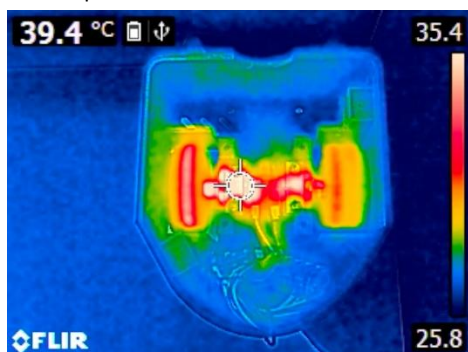
Figure 8. Temperature distribution during extreme load test of DC motors
