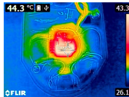
Figure 10. Temperature distribution during electronics extreme load test
