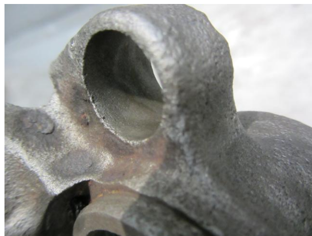
Figure 4. Sample of insufficiently cleaned component
