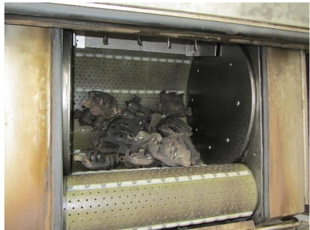
Figure 2. Wash machine for wet blasting
