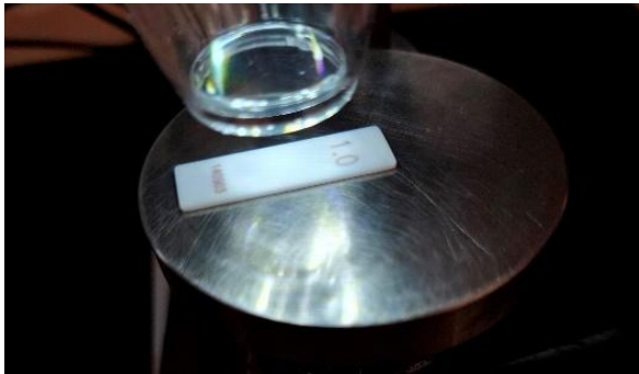
Figure 8. Measuring chamfer of gauge blocks.
