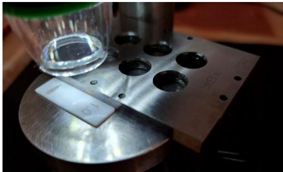
Figure 6. Visual inspection of the surface of gauge blocks
