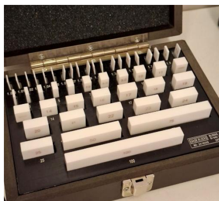
Figure 2. Gauge block set in wooden case (47-pieces)
